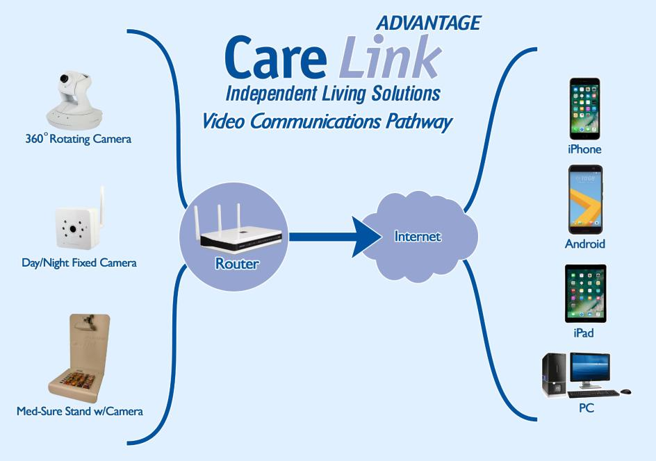
Cameras require an AC power connection and communicates wirelessly with the router
